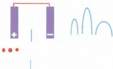
The count principle of the instrument is based on the measurement of changes in electrical resistance produced by a blood cell passing through an aperture sensor. Passing through the magnification circuit, the voltage signal will be magnified, which will be derived into impulses, and then analytical histogram will be generated.
